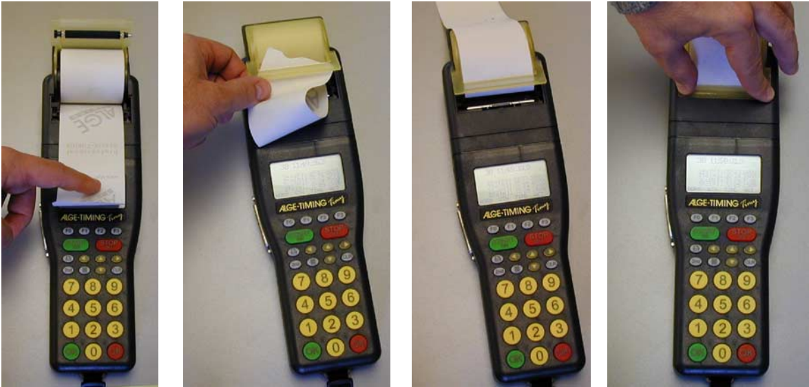
insert the new paper roll, so that the paper comes out in the front
